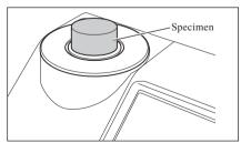
4. Make sure that 🕏 (Ready to measure) is displayed or the Ready lamp is green, and then press the measuring button.
