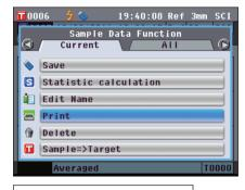
2. Press the [OK/Edit] button. The <Print Sample Data> screen is displayed and the data is printed out from the connected printer.
