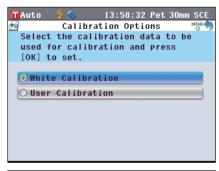
4. Use the ♠ or ♠ button of the cross key to move the cursor to "User Calibration" and then press the [OK/ Edit] button.
