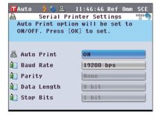
4. To change the baud rate, use the ♠ or ♠ button of the cross key to move the cursor to "Baud Rate" and then press the [OK/Edit] button.
