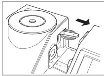
3. Block the receiving window of the Transmittance Specimen Chamber so that no dust or dirt enters through it.
