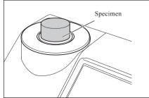
3. Make sure that \$\frac{1}{2}\$ (Ready to measure) is displayed and then press the measuring button.
