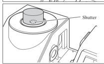
4. Look into the Specimen Viewing Mirror from the Top and adjust the position of the specimen.
