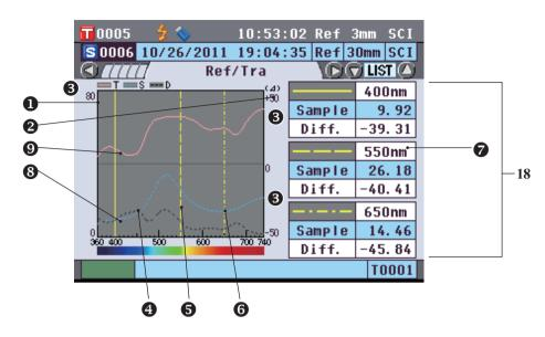
18 Sample data (The tab can be switched with the **①** or **②** button of the cross key.)
